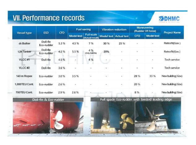
Below you can see the comparison between Doll-Fin & Eco-Rudder and Mewis Duct. It is obvious that the cost of the installation is much lower in these devices than the Mewis Duct device.
