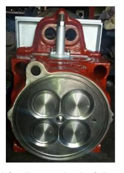
Original spare parts have been used for the overhaul of the cylinder heads.
